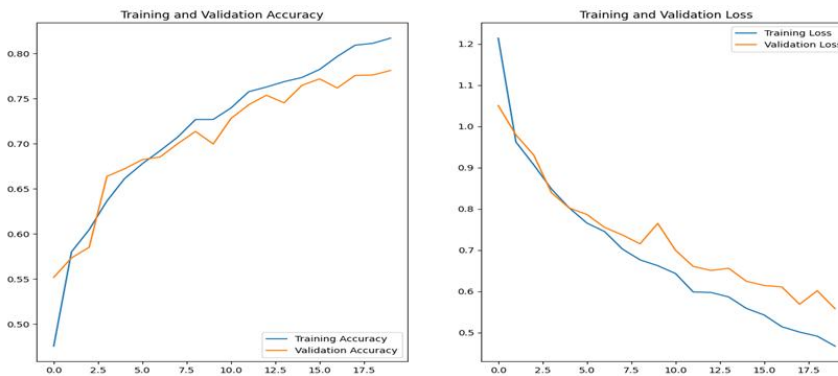
Fig. 16. Training & Validation Accuracy and Loss (VGG16)
