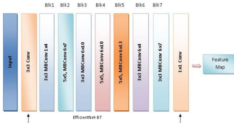
Fig. 4. The Architecture of EfficientNet-B7
